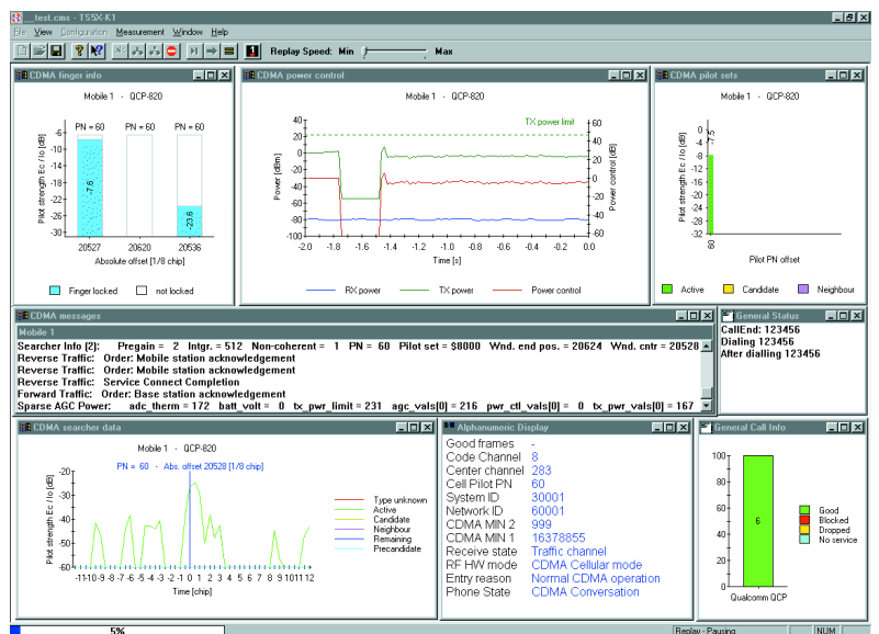
Coverage Measurement Software ROMES with various CDMA measurement displays
